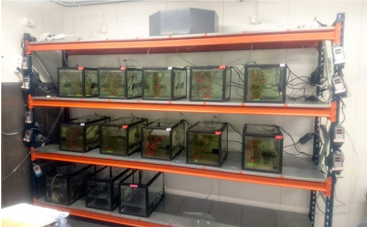
Fig S1. Experimental setup. The picture shows the tanks used in this experiment. Red labels indicates 34°C treatment and white label indicates 22°C treatment. The temperature in each tank is controlled with a thermostat (seen on the shelves columns) connected to one or two titanium heaters (seen on tank's left side). Each tank was equipped with one red and green ornamental plastic plant and two sponge biofilters for filtration, aeration and circulation. The 34°C tanks had an extra air stone installed to increase circulation over their heaters, resulting in a more even and stable temperature in their tanks.
