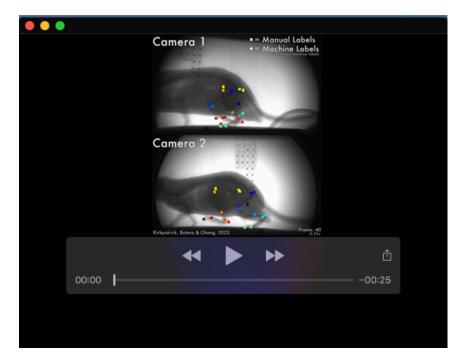
**Movie 1.** Example comparison of manual and machine labeled frames for a complete gait cycle. Unfiltered machine labels (marked with x) compared to manual labels (marked with a dot). Landmarks in this gait cycle were used to compute the joint angles in Fig. 3A. Label colors are consistent with the locations identified in Fig. 2A. X-ray video recorded at 100 fps and played back once at 1.0x speed, then twice at 0.25x for clarity.
