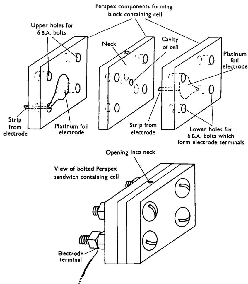
Fig. 4. Details of construction of a conductivity cell.
