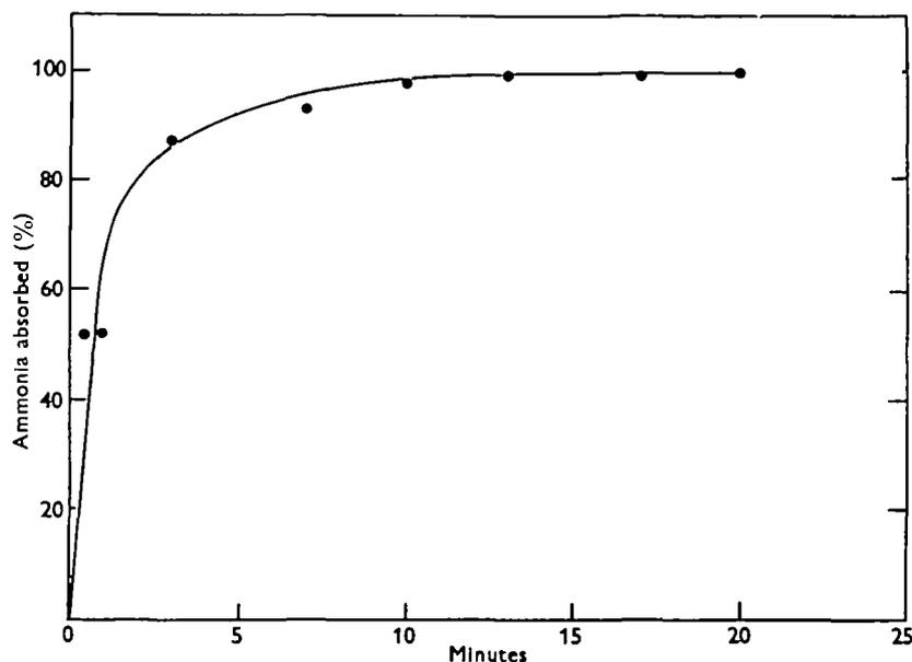
Fig. 3. The time course for the diffusion of ammonia (8.3 m $\mu$ g. ammonia-N) into 1.48  $\mu$ l. of 0.5 m.-equiv./l. H<sub>2</sub>SO<sub>4</sub>.
