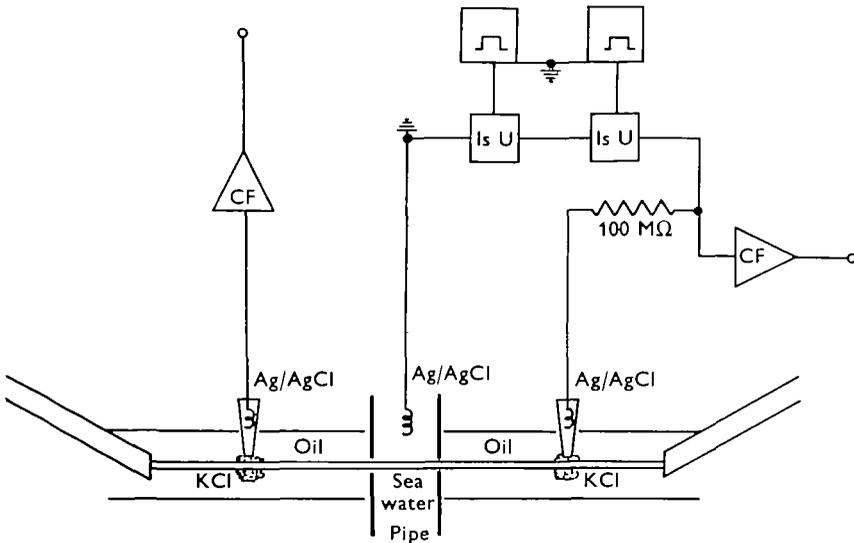
Fig. 1. Schematic diagram of the stimulating and recording system employed. Abbreviations: Ag/AgCl, silver-silver chloride; CF, unity gain cathode follower; Is U, stimulus isolation unit; KCl, isotonic potassium chloride Agar wick electrodes.
