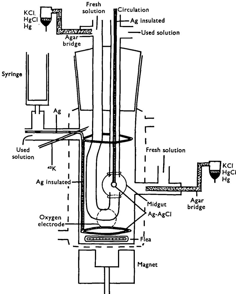
Fig. 2. Chamber used to perfuse the isolated midgut and measure the midgut potential, short-circuit current, K-influx and oxygen uptake (after Harvey *et al.* (1967)).  $^{42}\text{K}$  was injected through the cannula. Aeration and stirring of the lumen solution was accomplished through the upper ends of the lumen chamber. Broken lines indicate position of water jacket to maintain constant temperature.
