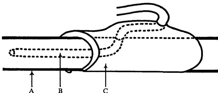
Fig. 3. Intra-aortic cannula: A, ventral aorta; B, polyvinyl tube; C, rubber jacket.
