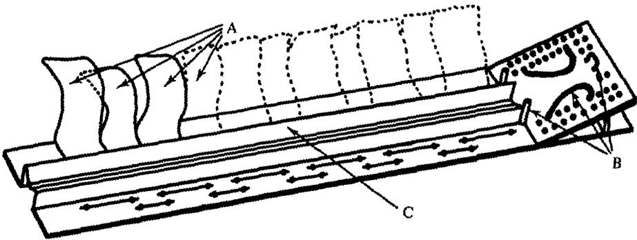
Fig. 1. Operating table: A, rubber retention bands; B, head retention apparatus; C, groove to retain body.
