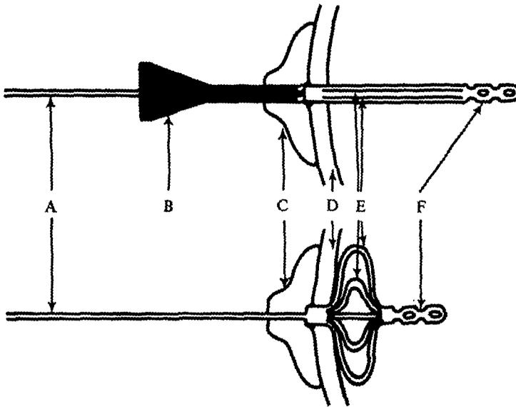
Fig. 2. Intra-bulbus cannula: above, before anchoring; below, cannula in position. A, Blood catheter; B, hypodermic needle; C, joint; D, wall of bulbus arteriosus; E, longitudinal lamellae; F, distal strainer.
