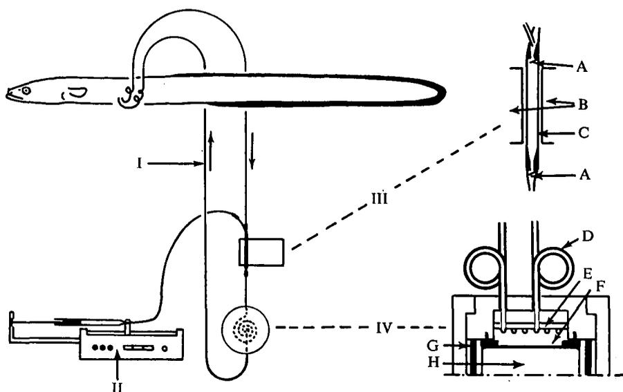
Fig. 5. Extra-corporal blood circuit: I, blood catheter (polyvinyl); II, perfusion syringe with heparinized solution; III, artificial heart; IV, counting device; A, unidirectional micro-valve; B, magnet; C, pulsing tube; D, opaque catheter; E, polyethylene joint; F, counting cell (SPF. La Radiotechnique); G, antimagnetic screen; H, Photo-multiplier tube.
