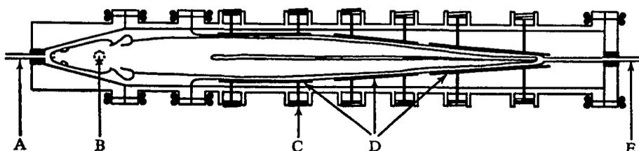
Fig. 4. Experimental tank seen from above: A, water entry; B, joint for exit of the extracorporeal blood tube; C, regulating screw; D, retention apparatus; E, water exit.
