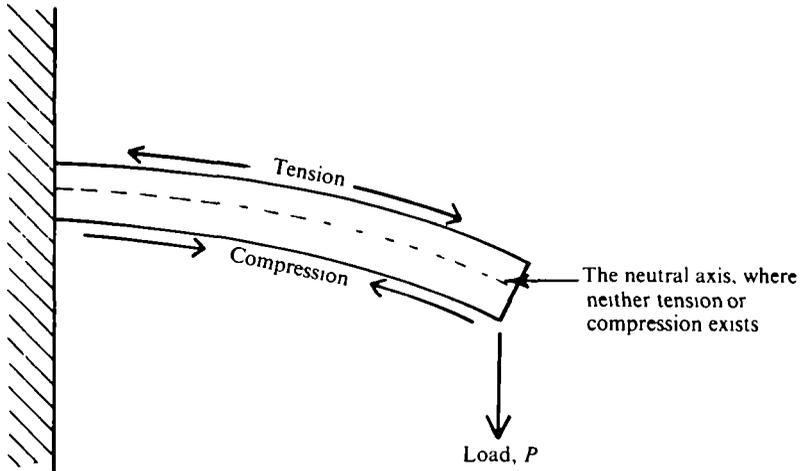
Fig. 1. Bending of a cantilever. A feather is structurally a cantilever, the base being inserted into the skeleton of the wing.
