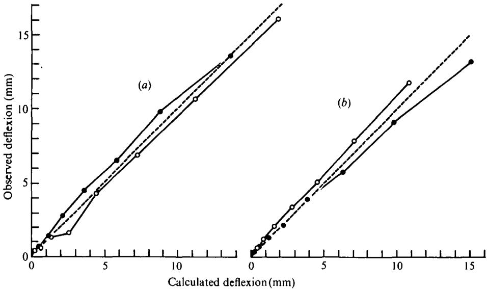
Fig. 7. Comparison between observed and calculated deflexions using equation (3) for the outermost feather (a) and the feather immediately proximal to it (b). The dotted line shows the line of perfect fit. Values of  $E$  used were: (a)  $7.75 \times 10^9 \text{ Nm}^{-2}$ ; (b)  $10^{10} \text{ Nm}^{-2}$ .  $\circ$  = dorso-ventral bending;  $\bullet$  = lateral bending.
