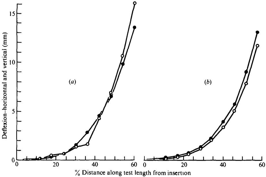
Fig. 6. Deflexions under static load applied at distances along the shaft for (a) the outermost feather and (b) the feather immediately proximal to it from the right wing of the 300 g bird. ○ = dorso-ventral bending; ● = lateral bending.
