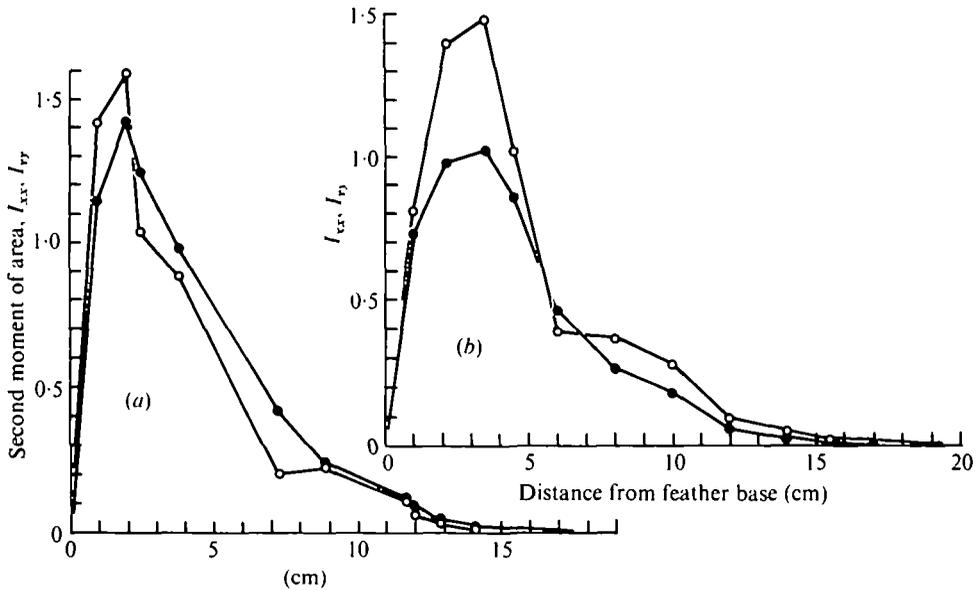
Fig. 5. Second moment of area values at distances along the shaft for (a) the outermost feather and (b) the feather immediately proximal to the outermost feather on the left wing of the 300 g bird.  $\circ$  =  $I_{xx}$  values;  $\bullet$  =  $I_{yy}$  values.
