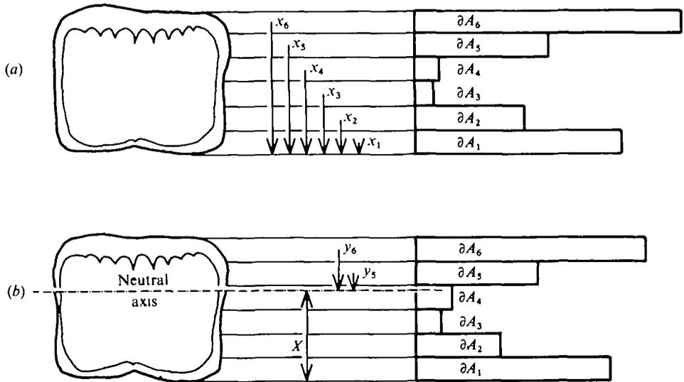
Fig. 2. (a) First moment of area calculation. The cortex is divided into strips. The area of cortex in each strip,  $A_i$ , and the distance ( $x_i$ ) of the centroid of each area from an arbitrary baseline is measured. (b) Second moment of area calculation. The position of the neutral axis is taken from the first moment of area. The distance from the neutral axis to each centroid of area,  $y_i$  is measured.
