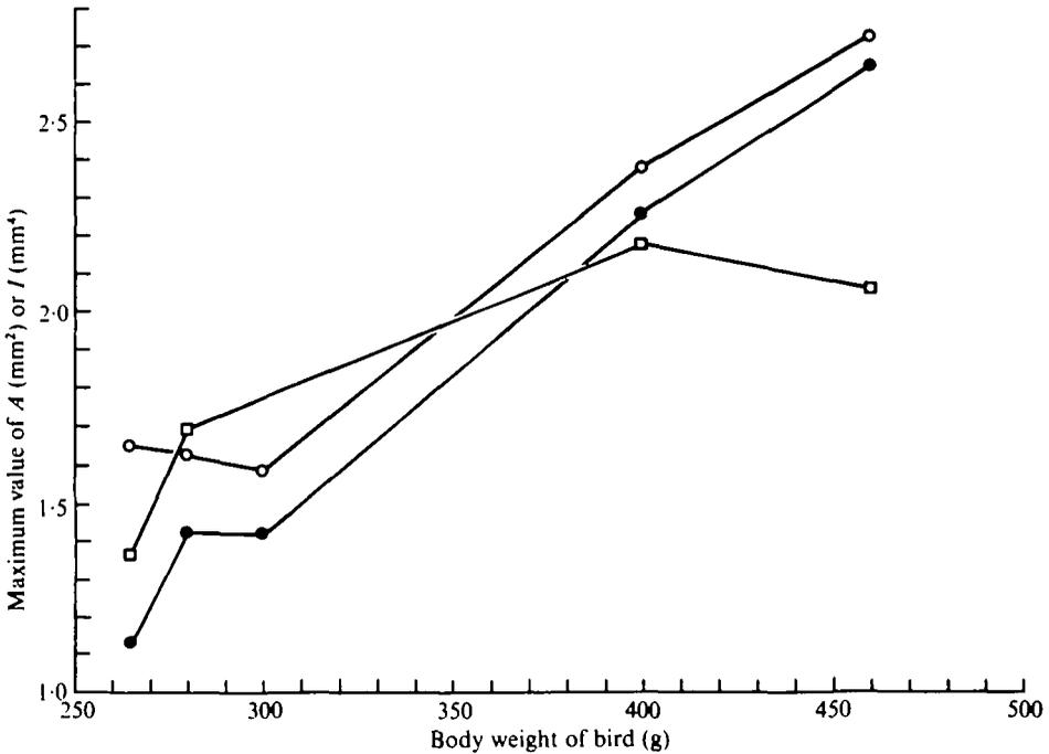
Fig. 8. Maximum  $I$  values and maximum area of cortex found in the shaft *v.* body weight of bird. ○ =  $I_{zz}$  max; ● =  $I_{yy}$  max; □ =  $A_{max}$ .
