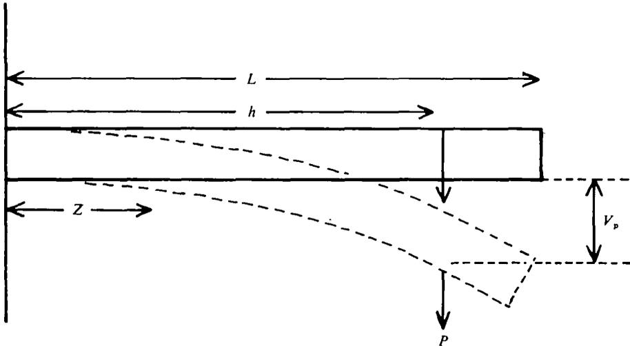
Fig. 3. Deflection in a cantilever beam under static point load.
