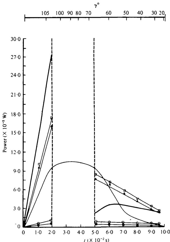
Fig. 9. The power required to accelerate and decelerate the added mass of the fin ( $\square$ ), its individual blade-elements ( $e_2$  ( $\blacksquare$ ),  $e_3$  ( $\circ$ ),  $e_4$  ( $\blacktriangle$ ), the total power required to produce the hydrodynamic thrust force (thin solid line) and the total power needed (heavy solid line) are plotted against time.
