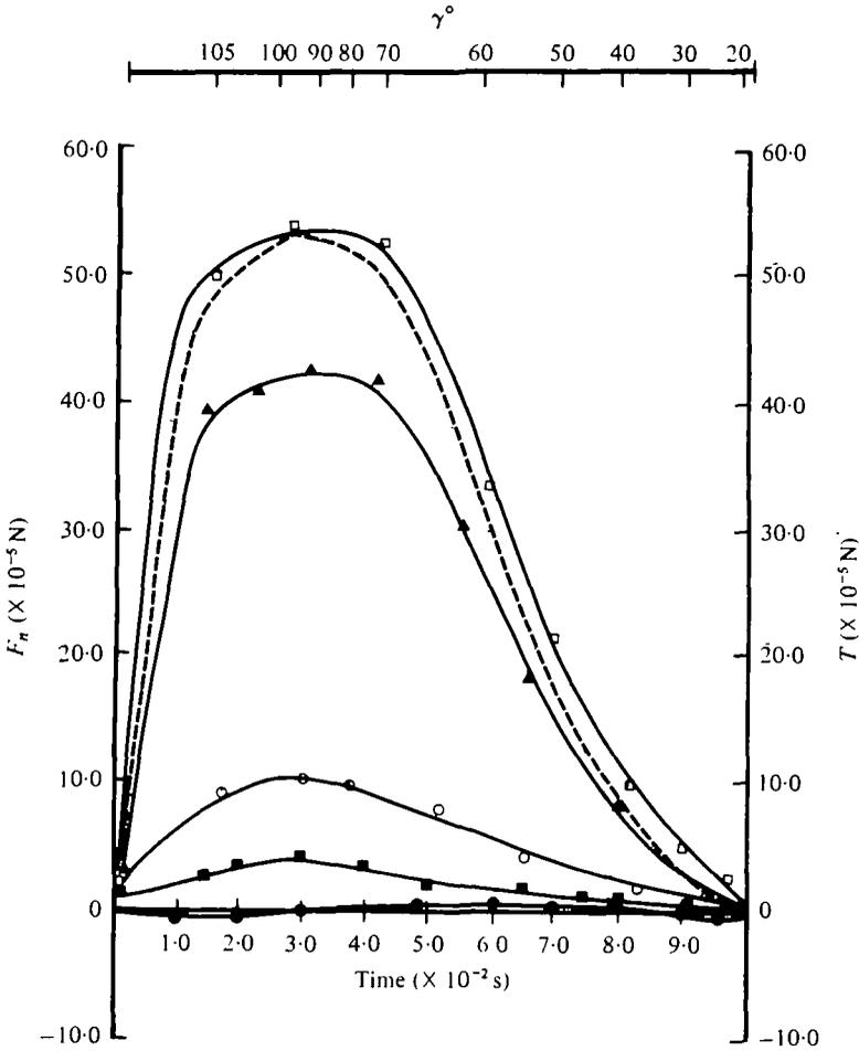
Fig. 6. The normal force acting on the elements (●, e<sub>1</sub>; ■, e<sub>2</sub>; ○, e<sub>3</sub> and ▲, e<sub>4</sub>), the total force (□) and the total thrust (broken line) acting on the elements during the power stroke are also shown.
