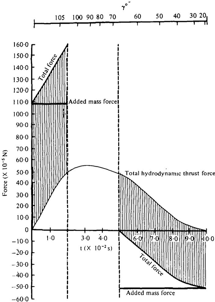
Fig. 8. The total hydrodynamic thrust force, added mass force and total force acting on the fin is plotted against time. The accelerations occurring between  $t = 2.0 \times 10^{-2}$  s and  $t = 5.0 \times 10^{-2}$  s are small and could not be measured accurately. The impulse of the added mass force is indicated by the shaded area.
