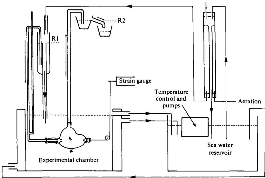
Fig. 2. Diagram of the experimental apparatus used to maintain and perfuse physiological preparations. The input pressure to the isolated ventricle was set by adjusting the height of reservoir  $R_1$ . The output back pressure was set by the height of the reservoir  $R_2$ . The arrows indicate the direction of flow. The component parts of this set-up are not drawn to scale.
