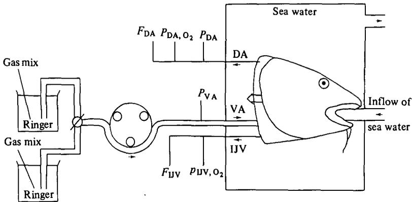
Fig. 1. Schematic representation of the perfusion arrangement. Details are given in the text. DA, Dorsal aorta;  $F_{DA}$ , dorsal aorta flow;  $F_{IJV}$ , inferior jugular vein flow; IJV, inferior jugular vein;  $P_{DA}$ , dorsal aorta pressure;  $P_{DA,O_2}$ , dorsal aorta effluent  $p_{O_2}$ ;  $P_{IJV,O_2}$ , inferior jugular vein effluent;  $p_{O_2}$ ,  $P_{VA}$ , ventral aorta pressure; VA, ventral aorta.
