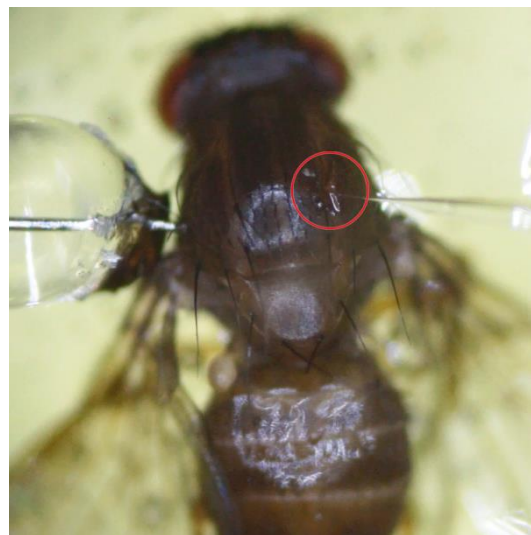
Fig. S1. Photo showing the placement of the electrodes. The reference electrode were inserted directly through the carapace (left) and glass electrode inserted into a flight muscle through a small window in the carapace cut with the tip of a syringe-needle (circled).
