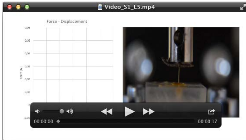
Movie 1. The onset and evolution of local buckling in a tibia specimen at the fifth nymphal stage (L5).
